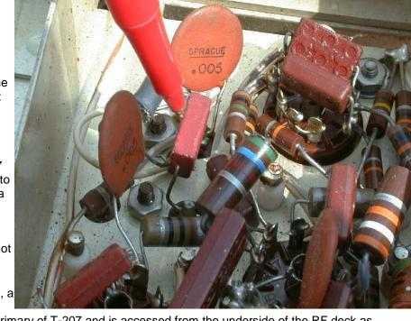
This is caused by C-327, a 100pf mica capacitor
