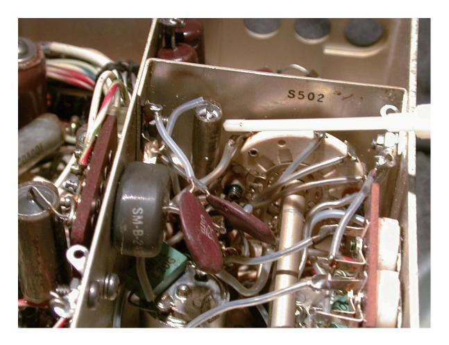
Remove the old C-553 and install a .01ufd, 600V Sprague Orangedrop capacitor in its place. Try and nest it vertically in the chassis as original. Because B+ is involved, be sure to use shrink tubing fully covering any exposed leads on the new capacitor.
